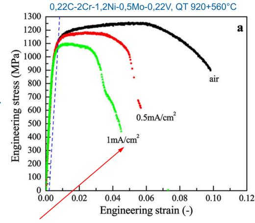
Low ductility with hydrogen in steel
